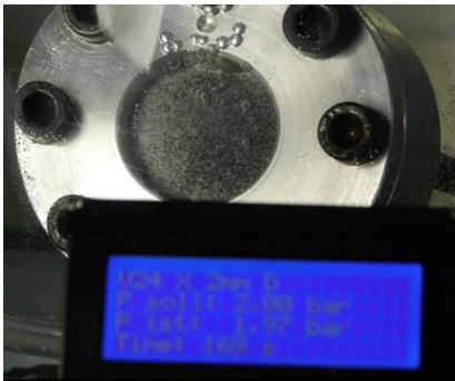
Test set-up for measuring air tightness
